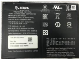
BTRY-ET5X-10IN5-01 10 in. Tablet Internal Battery
