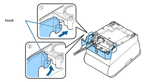
3. Push the connector cover down to click onto the printer case.
